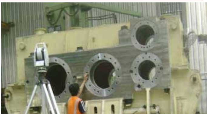
LASER TRACKER ON A GEARBOX CASING
