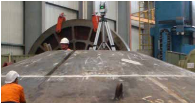
LASER TRACKER ON A MILL HEAD
